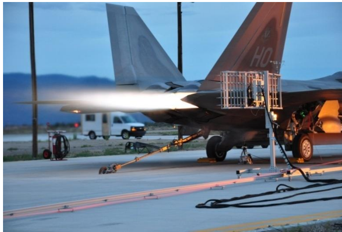
Figure 3.2 Blue Ridge Research and Consulting 90-microphone array, scanning the near field of the jet on an F-22 Raptor.
